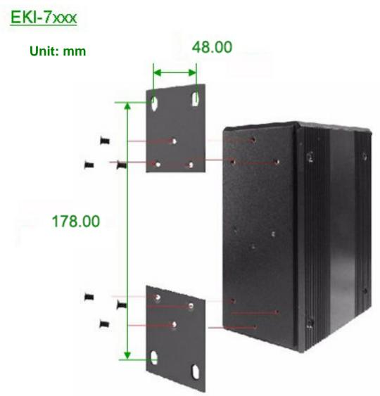
Figure 2.3-1 Combine the Metal Mounting Kit
