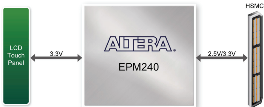
Figure 3-6 Block Diagram of the Bus Controller
