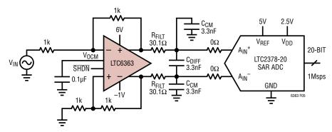
Figure 5. Recommended Interface Solution for Driving the LTC2378-20 SAR ADC
