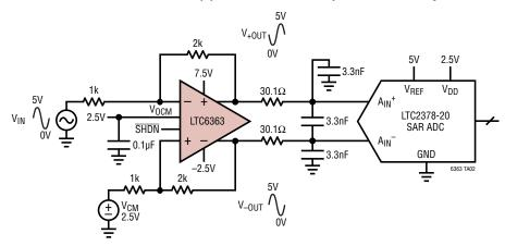
Differentially Driving an ADC with  $\Delta V_{IN}$  = 10V  $_{P\text{-}P}$  and Gain of  $A_V$  = 1
