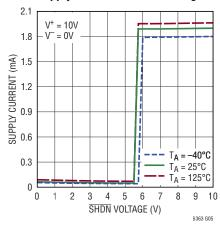
Shutdown Supply Current vs Supply Voltage
