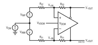
Figure 3. Real-World Application with Feedback Resistor Pair Mismatch
