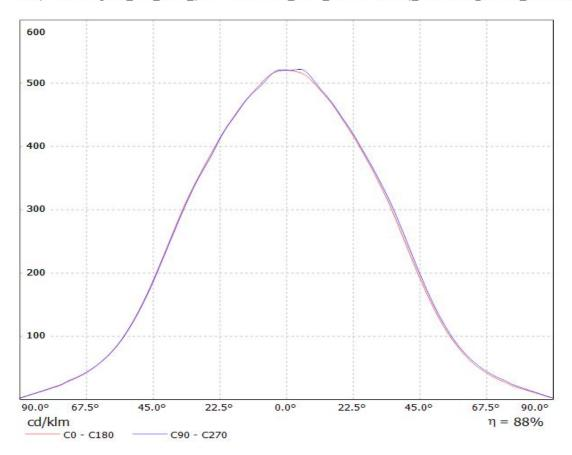
Luminaire: Ledil Oy FN15737\_RONDA-WWW-B\_BRIDGELUX\_V10\_Gen7\_SIMULATED Lamps: 1 x BRIDGELUX V10 Gen7
