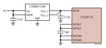
Figure 8. Using the LTC6655-2.048 as an External Reference
