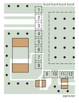
Figure 7. Suggested REFBUF Bypass Capacitor Layout
