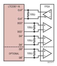
Figure 11. Digital Output Interface to an FPGA
