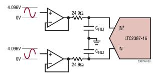
Figure 3. Typical Input Drive Circuit
