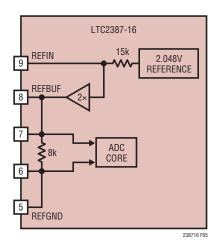
Figure 5. LTC2387-16 Internal Reference Circuitry
