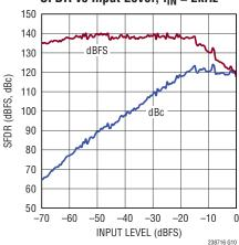
SFDR vs Input Level,  $f_{IN} = 1MHz$
