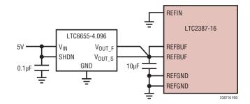
Figure 9. Overdriving REFBUF Using the LTC6655-4.096
