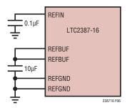
Figure 6. Configuration for Using the Internal Reference
