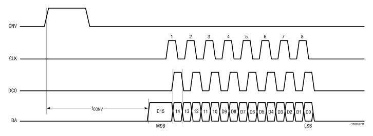
Figure 12. Timing Diagram for a Single Conversion in One-Lane Mode
