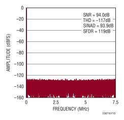
Figure 10. 32k Point FFT of the LTC2387-16, f<sub>SMPL</sub> = 15Msps, f<sub>IN</sub> = 2kHz
