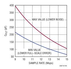
Figure 4. Suggested Range of CFILT Values vs Sample Rate
