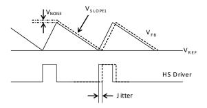
Figure 4—Jitter in PWM Mode
