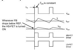
Figure 2—Heavy Load Operation
