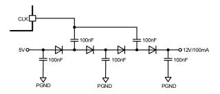
Figure 7—Charge Pump Circuit
