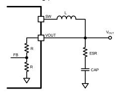
Figure 6—Simplified Circuit in PWM Mode
