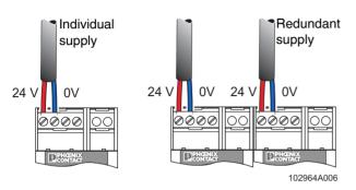
Figure 9 Individual/redundant supply
