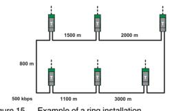
Figure 15 Example of a ring installation
