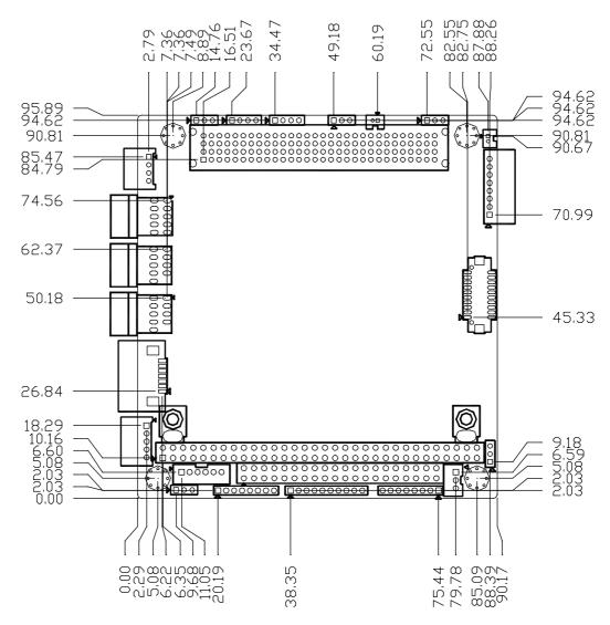
Figure 1.1 Board layout: Dimensions (Component Side)
