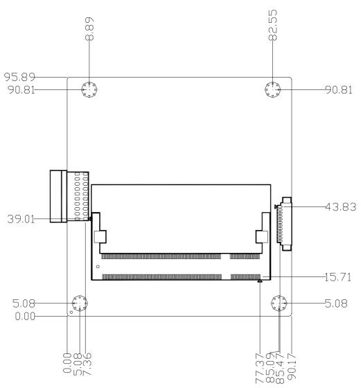
Figure C.2 PCM-3362 Mechanical Drawing (Solder Side)
