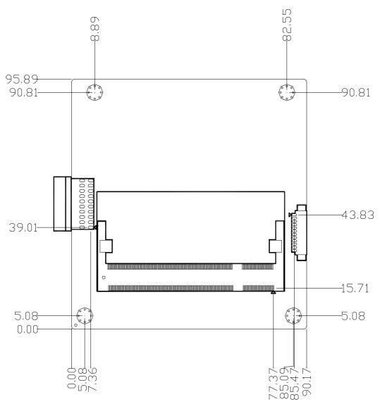
Figure 1.2 Board layout: Dimensions (Solder Side)
