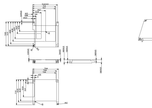
Figure C.5 PCM-3362 optional Heatspreader Mechanical Drawing
