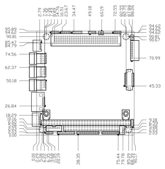
Figure C.1 PCM-3362 Mechanical Drawing (Component Side)
