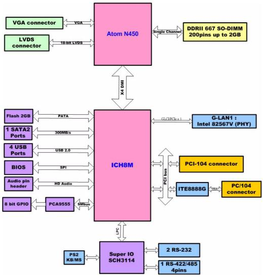
Figure 2.3 Block diagram
